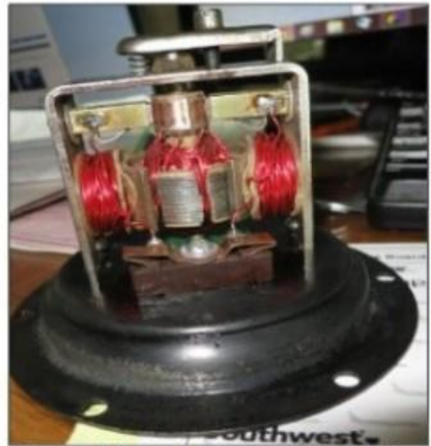
Rewound field and armature by Steve Smith
