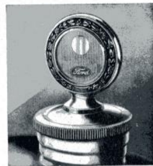
Fig. 538—Radiator Cap with Motometer
