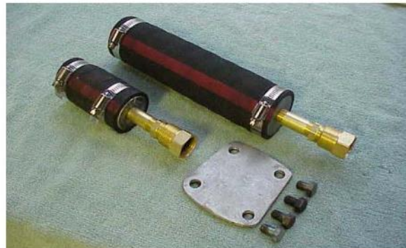
Shown above are the two adapters and the water pump blanking plate. The long hose is the upper (larger diameter) hose. The short hose is the lower (smaller diameter) hose.
