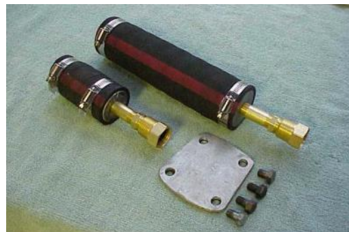
Shown above are the two adapters and the water pump blanking plate. The long hose is the upper (larger diameter) hose. The short hose is the lower (smaller diameter) hose.
